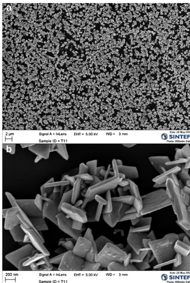
**Fig. 3** Sample t11b, deposited with 10 mM NaOH at 0.9 V **a** overview and **b** detail. Scale bars are 2  $\mu\text{m}$  and 200 nm
