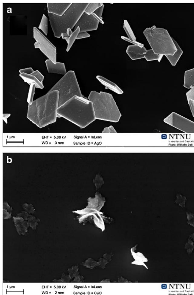
**Fig. 1** Deposition from individual nitrates. **a** Platelets of AgO and **b** clumps of copper oxides/hydroxides. Scale bars are 1  $\mu\text{m}$
