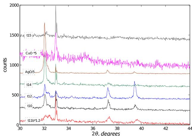
**Fig. 5** X-ray diffraction results for films deposited at different pH and applied voltage. (Color online) Peak amplitudes (as indicated) and base-lines have been adjusted to improve readability
