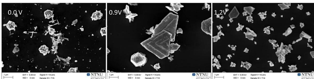
**Fig. 4** Samples deposited at 0, 0.9, and 1.2 applied volts using 25 mM NaOH. Scale bars are 1  $\mu\text{m}$
