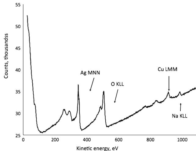
**Fig. 6** Auger survey scan for a particle on sample t10, dominated by oxygen, silver, and copper peaks
