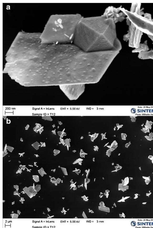
**Fig. 2** Sample t12, deposited with 25 mM NaOH at 0.9 V **a** detail and **b** overview. Small deposits (bumps) are residual NaOH. Scale bars are 200 nm and 2  $\mu\text{m}$
